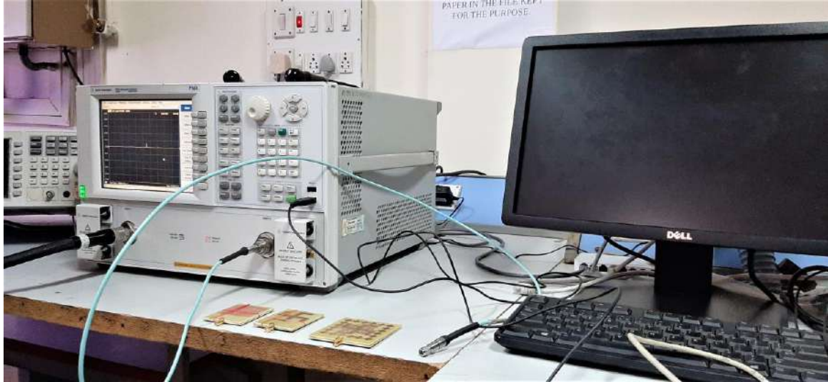
Figure 6.1 Testing for return loss
