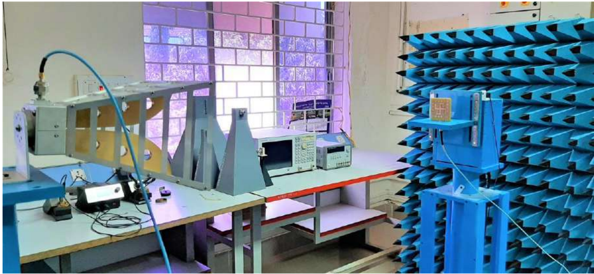
Figure 6.2 Testing for gain
